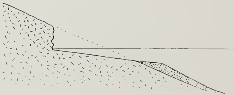
FIG. 27.—Cross-section of a wave-cut cliff and its accompanying cut-and-built terrace. (Illinois Geol. Survey Bull. 7, fig. 20, 1908).
